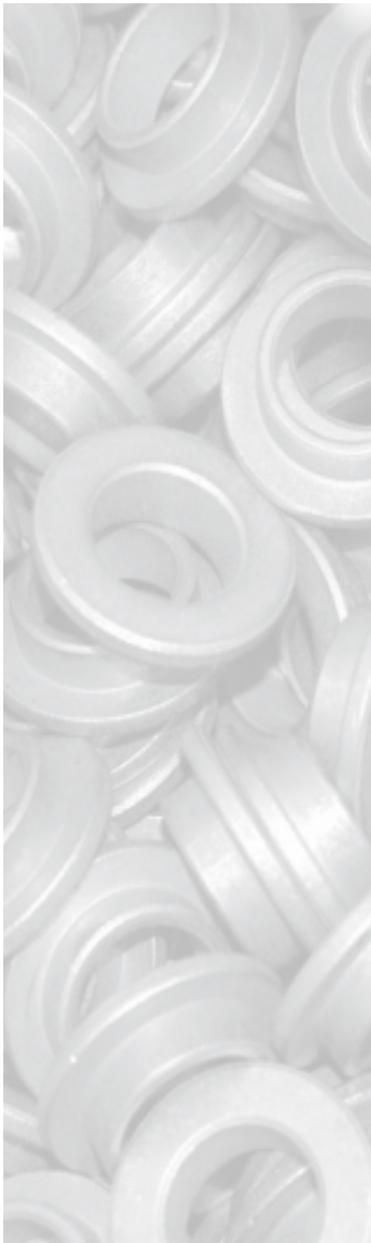
Sintered powdered metal or “porous” bearings, which are impregnated with lubricating oil through a vacuum process, are generally used as an alternative to expensive rolling element bearings. In addition to impregnation, a small reservoir, usually an oil-soaked felt pad, is sometimes placed adjacent to the bearing to augment oil supply and thus extend bearing life.
