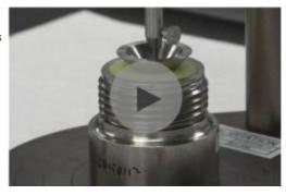
area that needs to be lubricated in an application. The Po, or unworked and P60 or worked penetration tests follow ASTM D-217 method for full scale or ASTM D-1403 method for half scale or quarter scale.
