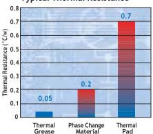
Compared to thermal pads and phase change materials, thermal grease offers the lowest possible thermal resistance.
