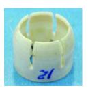
Results after 82,500 Cycles. Ball joint on the left was lubricated with fortified petroleum grease. Ball joint to the right and plastic bearing insert were lubricated with Nye's Fluorocarbon Gel 880. Ball joints are shown after 82,500 cycles under the same test conditions. (Photos Courtesy: Dana Industrial Ltda.)
