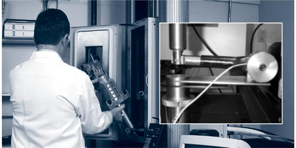
*Nye has used the Instron 5566 to pre-qualify lubricants for master cylinders, steering columns...and now for ball joints (inset). The Instron performs tensile, compression, shear, peel, tear, flexural, and other tests on a wide variety of materials and components.*
