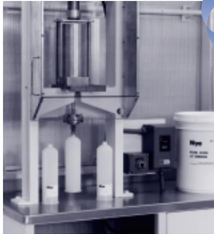
*One of four Class 100 MIN environments recently installed at Nye.*
